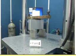
10. Mechanical Shock Test: +Y axis
