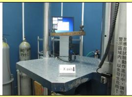
9. Mechanical Shock Test: -X axis
