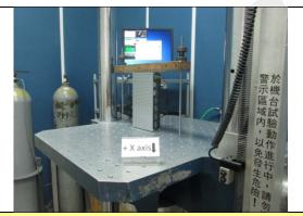
8. Mechanical Shock Test: +X axis
