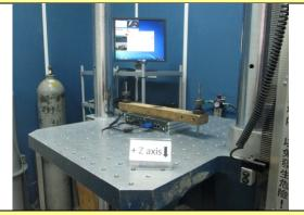
12. Mechanical Shock Test: +Z axis
